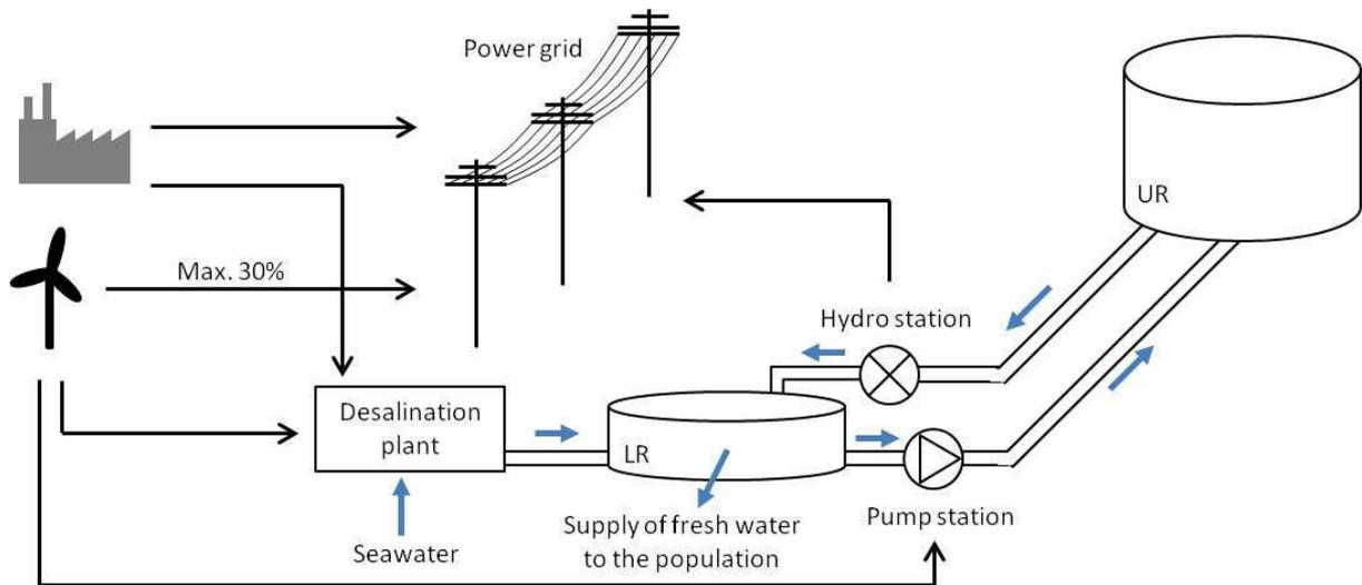
Figure II.12 - Schematic diagram the wind powered desalination and PHS system.
