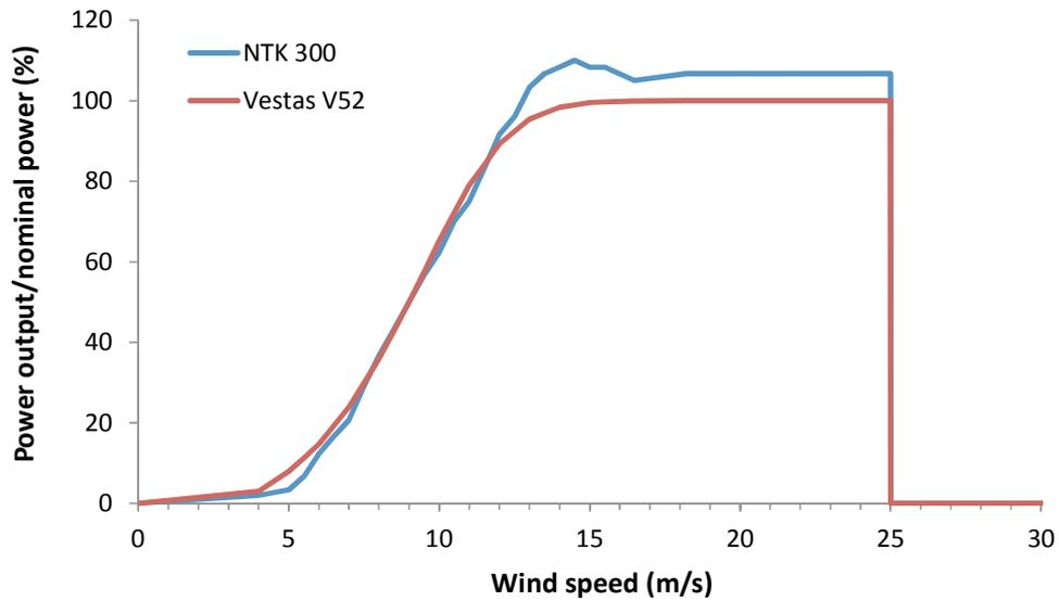
Figure II.4 – Wind power curve of the wind turbines installed in S. Vicente [85,86].
