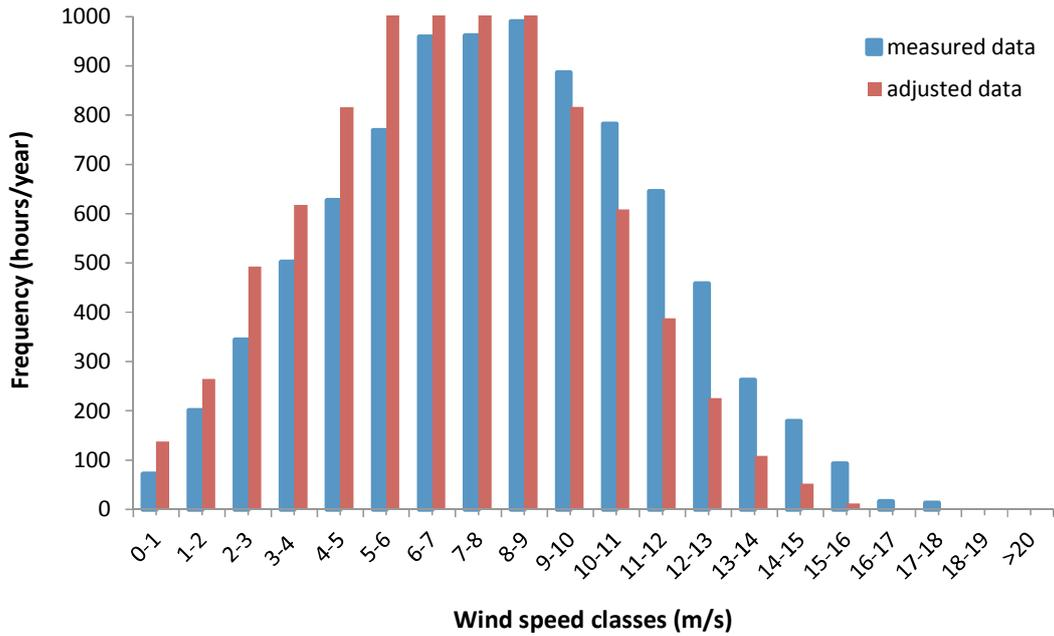
Figure II.8 – Frequency of occurrence of measured and adjusted wind speed in 2005.
