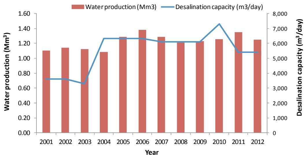
Figure II.9 - Water production and desalination capacity installed in S. Vicente from 2001 to 2012 [14,73-83].
