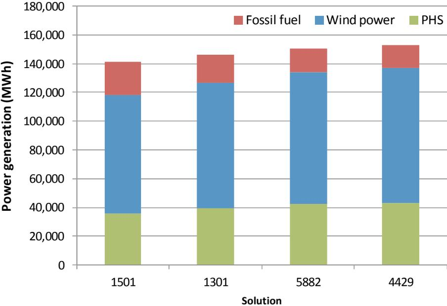
Figure IV.11 - Power generation for each solution analysed.
